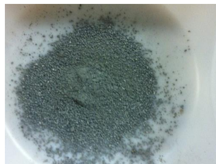
Figure 5. Spent FeOx/n-ZrO 2 catalyst after 10 cycles.
