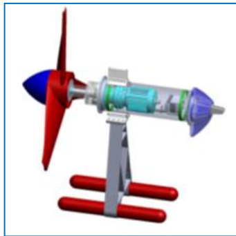
Figure 2. SNMREC 3-Meter Diameter Rotor, 20kw Instantaneous Max Power Prototype Turbine
