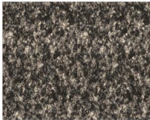
Structure of the porous nanoparticle of \text{TiO}_2 fabricated with the spraying system
