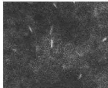
Structure of the PSDOT/PSS doped with ZnO nanoparticle fabricated with the spin coating system
