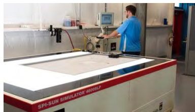
Figure 1: PV module testing with flash simulator
