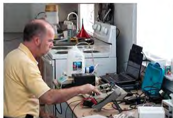
Project Specialist, David Hoak calibrates schedule controller to use with latent load generator.
