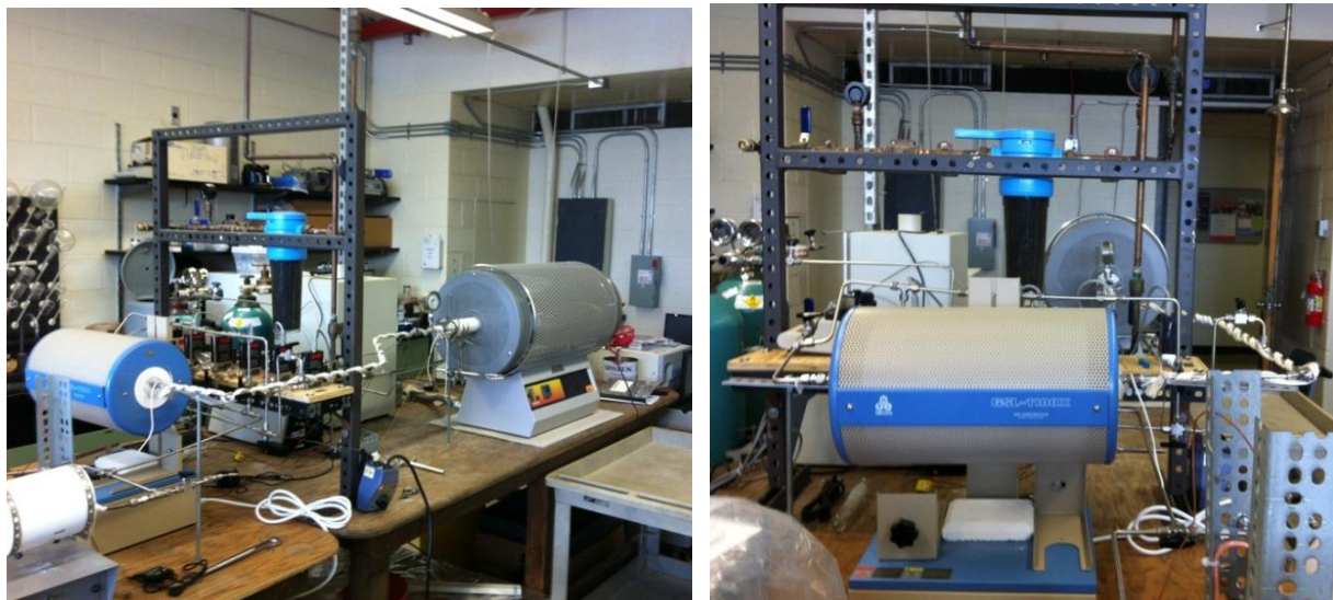
Figure 2: a) (left) Completed water-splitting reactor system, and b) (right) evaporator furnace used to produce steam for the water-splitting step.
