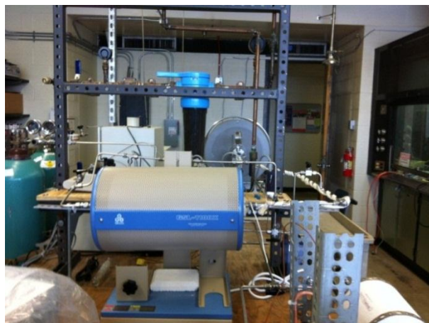
Figure 1. Top: drawing of reactor system. Bottom left: photo of syringe pump and evaporator. Bottom right: photo of high-temperature reactor (mass spectrometer for product analysis is visible in the right hand corner of the photo).
