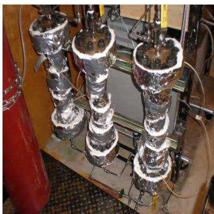
Figure 6: (left) Multistep filtrations setup (right) Total ion chromatogram of biomass derived syngas after cleansing.
