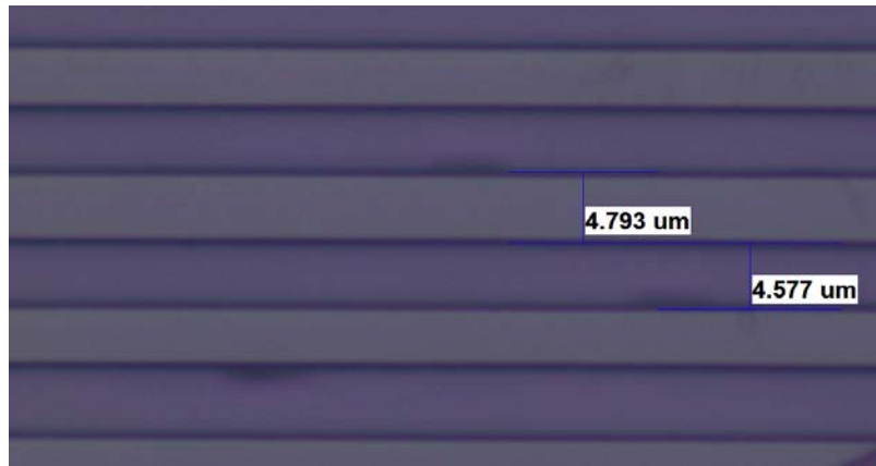
Figure 8. A micrograph of the fabricated plasmonic emitter with a depth of 2.7 microns and grating pitch of 9.3 microns.
