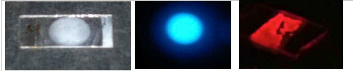
Fig. 7: (a) View of a device fabricated with nanoparticle coatings, (b) blue emitting device with La 2 O 3 :Bi phosphor, (c) red emitting device with CaS:Eu phosphor.
