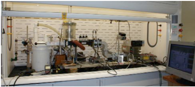
Fig. 4: Picture of the microwave plasma system used in the growth of nanophosphors, ZnO and ZnS layers.
