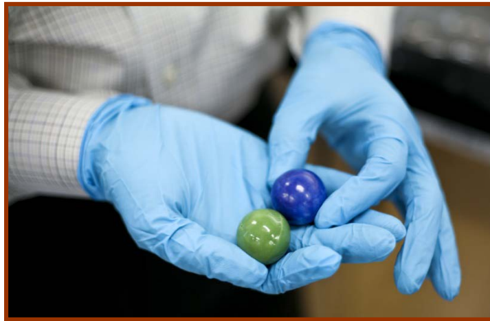
Figure 15 Ceramic encapsulated PCM for high temperature thermal energy storage
